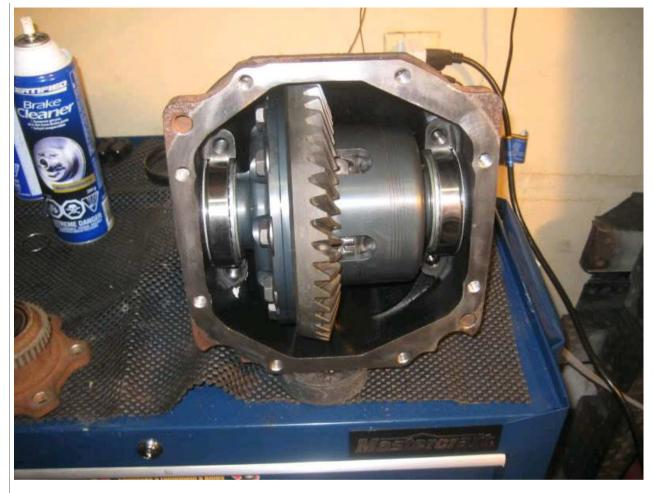
I placed the bearing caps on, and hand tightened the bolts. Then I torqued them in a criss cross pattern again to 65-72ft lbs.
