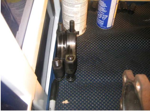
This was really tight (obviously) so I had to tap it out from the axle holes with a mallet and punch. Eventually I worked it out. If you care about your OEM VLSD then I would advise using brass drifts, or using a slide hammer to pull it out. I didn't care and you'll see later there is some damage on the inside from my use of cold steel punches.
