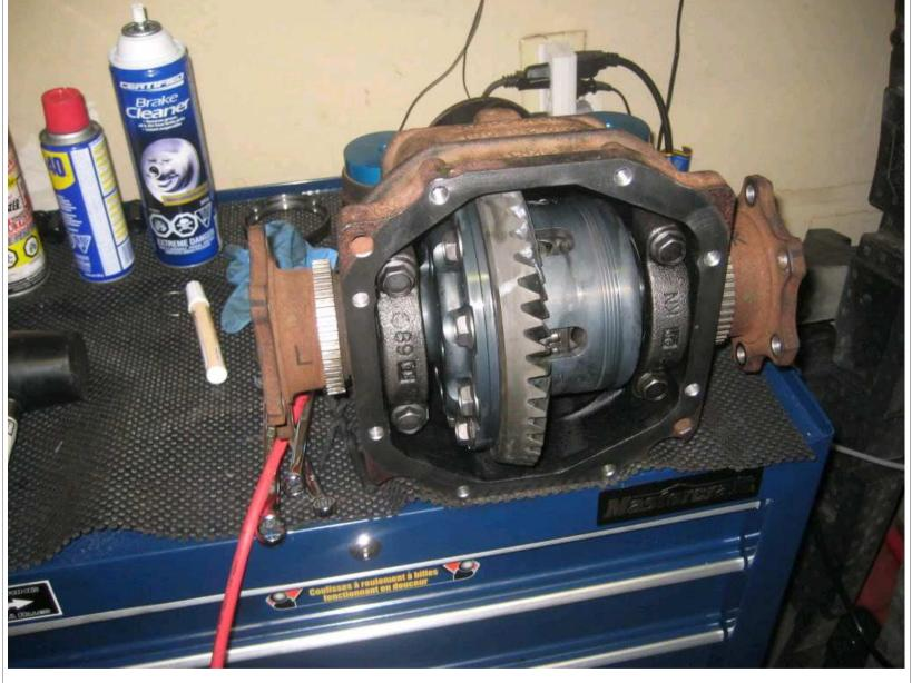
Using RTV high heat red, I made a gasket on the diff housing.
