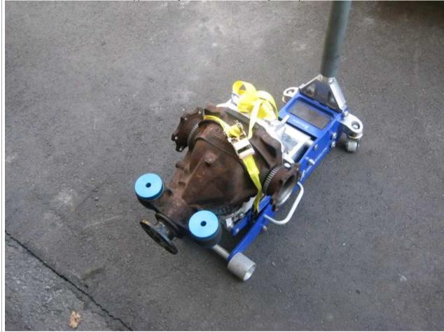
Oh to make my life a million times easier, something I should have taken the time to do in the beginning was remove the rear sway bar. This allows me to get directly under the car with the jack and lift it straight into place. With the sway in, I had to work it out over top...hindsight is 20/20, like a lot of things I learned during all of this.
