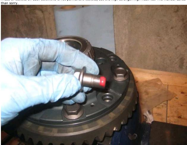
Torque in a criss cross pattern from 55ft lbs to 61ft lbs then turn them 30 degrees more according to the manual.
