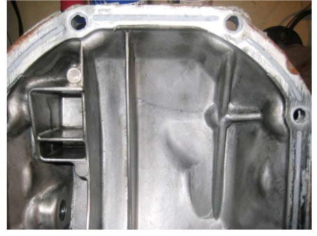
If I flip the cover around, that crack is stemming from where the rear sub frame mount is. But it's only on the inside...
