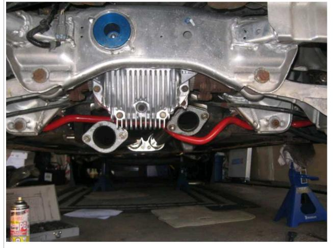
The most annoying thing was probably the rear HKS exhaust canisters, they are heavy and \*\*\*\*ing awkward, especially with the rubber bushings they connect to. PB Blaster on the bushing made them slide in really easy.
