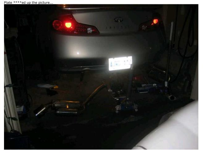
Over the past few days for about an hour a night, I was taking the diff itself out, unbolted exhaust, drive shaft, axle stubs, bushing mounts and dropped it out.
