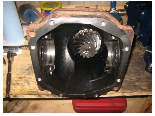
Place shims in appropriate locations with new bearing races.
