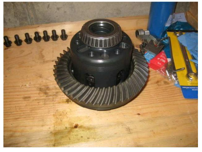
So at this point, Nissan recommends replacing all the ring bolt hardware and not re-using, I assume due to the stress on the bolts. I don't have them yet...so again it sits for now.
