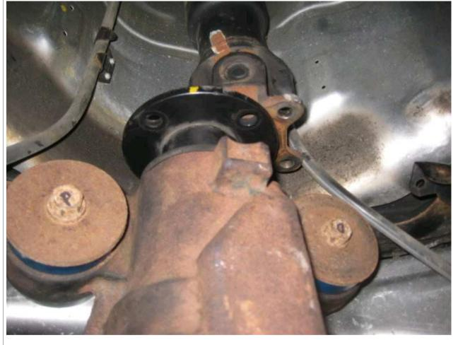
Torque the rear mount bolt to 74-88ft lbs and the 2 fronts to 67-81ft lbs, connect the wheel sensors.
